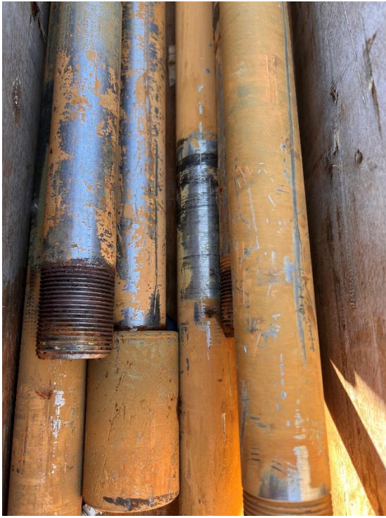
Photo #9: Another View of Line Shafts. Moderate Wearing Can Be Seen Where The Spider Bearing Bushings Sit on the Shaft.
