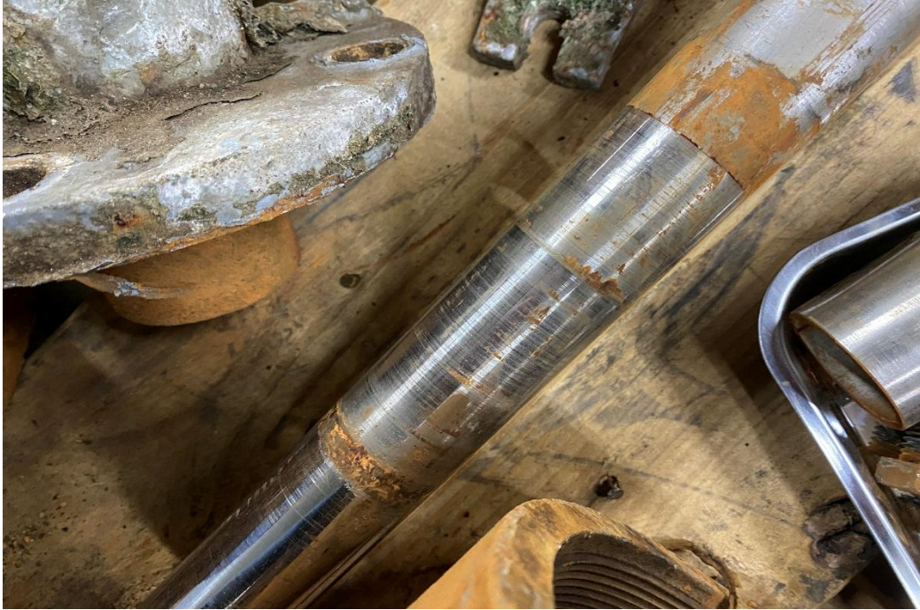
Photo 3: View of Pump Shaft, signs of heavy wearing
