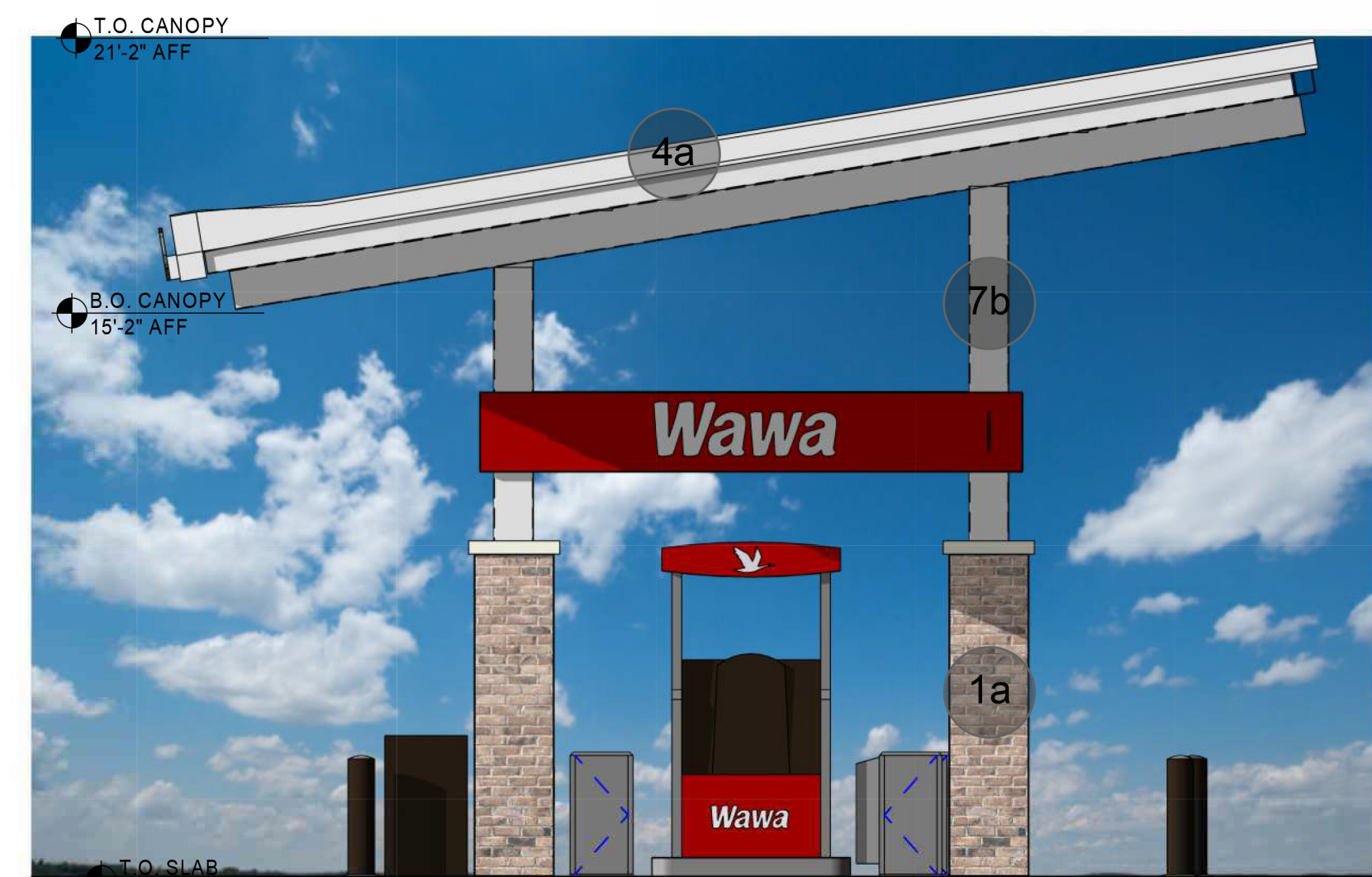
7 FUEL CANOPY ELEVATION 1/4" = 1'-0"
