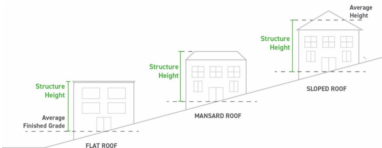
Figure 1150-1: Examples of how to measure building height
