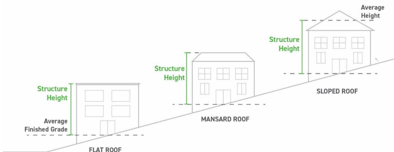
Figure 1150-1: Examples of how to measure building height
