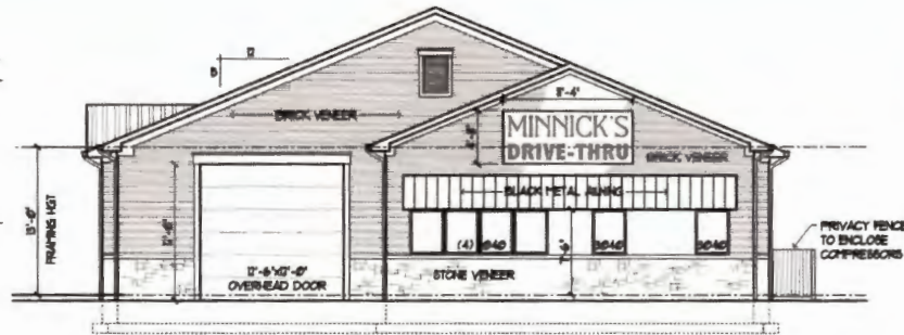
WEST (FRONT) ELEVATION 1/8" = 1'-0" FACING RIVER ROAD
